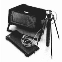
To improve performance while canceling unwanted sound, Flowmaster used a spectrum analyzer and a Super-Flow dyno incorporating an Engine Cycle Analyzer.
