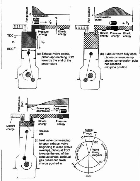
Cam overlap, intake manifold runner length, and exhaust design all affect how efficiently the spent gas vacates the cylinder bore.
