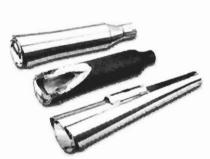
The SuperTrapp muffler allows the user to tune back pressure by adding or removing disks
