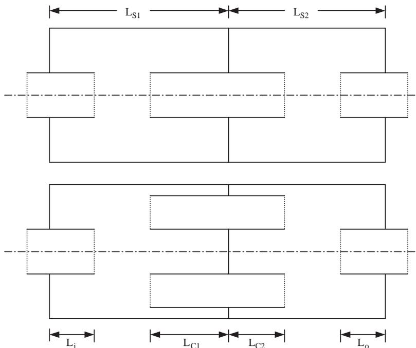
Fig. 1. Double expansion chamber silencers with single and double inter-connecting tubes.
