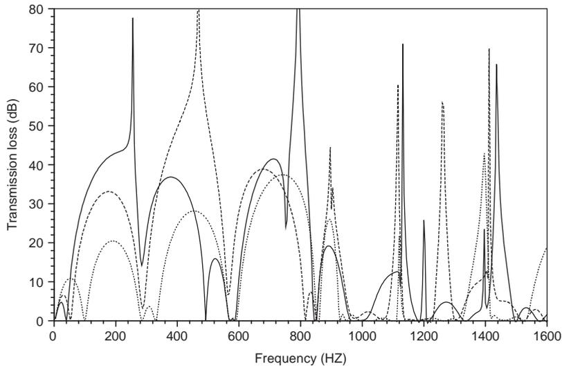
Fig. 4. Effect of length of inter-connecting tube on acoustic attenuation performance of double chamber silencer ( $L_{s1} = L_{s2} = 24''$ ): ———,  $L_{c1} = L_{c2} = 12''$ ; - - - - - ,  $L_{c1} = L_{c2} = 6''$ ; ·······,  $L_{c1} = L_{c2} = 0$ .
