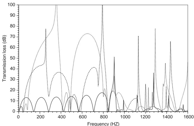
Fig. 3. Acoustic attenuation performance comparison of single and multiple expansion chamber silencers: ———, single chamber silencer ( $L_s = 48''$ ); - - - - -, double chamber silencer ( $L_{s1} = L_{s2} = 24''$ ,  $L_{c1} = L_{c2} = 12''$ ); ..... Triple chamber silencer ( $L_{s1} = L_{s2} = L_{s3} = 16''$ ,  $L_{c1} = L_{c4} = 8''$ ,  $L_{c2} = L_{c3} = 4''$ ).
