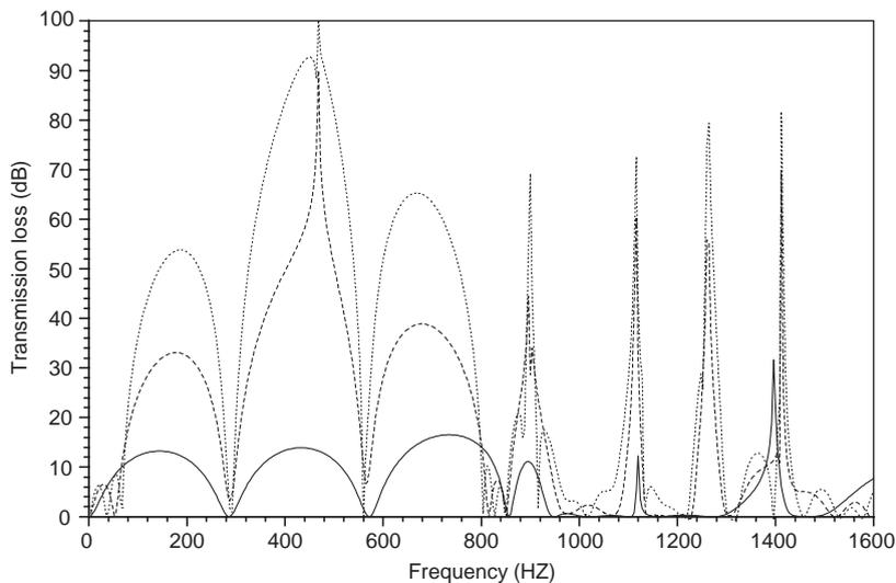
Fig. 2. Acoustic attenuation performance comparison of single and multiple expansion chamber silencers: ———, single chamber silencer ( $L_s = 24''$ ); - - - - -, double chamber silencer ( $L_{s1} = L_{s2} = 24''$ ,  $L_{c1} = L_{c2} = 6''$ ); ..... triple chamber silencer ( $L_{s1} = L_{s2} = L_{s3} = 24''$ ,  $L_{c1} = L_{c2} = L_{c3} = L_{c4} = 6''$ ).
