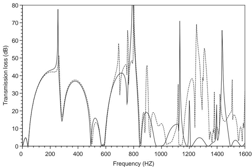
Fig. 7. Effect of the number of inter-connecting tube on acoustic attenuation performance of double chamber silencer ( $L_{s1} = L_{s2} = 24''$ ,  $L_{c1} = L_{c2} = 12''$ ): ———, single inter-connecting tube; ..... , double inter-connecting tubes.
