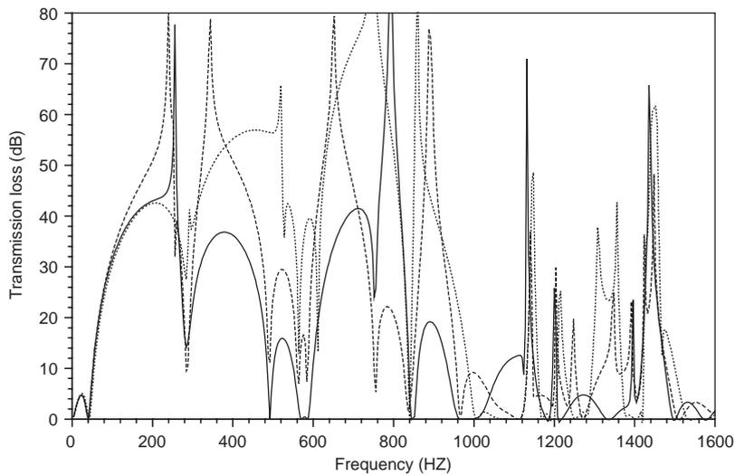
Fig. 6. Effect of extensions of inlet and outlet tubes into chambers on acoustic attenuation performance of double chamber silencer ( $L_{s1} = L_{s2} = 24''$ ): ———,  $L_{c1} = L_{c2} = 12''$ ,  $L_i = L_o = 0$ ; - - - - - ,  $L_{c1} = L_{c2} = 12''$ ,  $L_i = 7''$ ,  $L_o = 4''$ ; ..... ,  $L_{c1} = L_{c2} = 10.5''$ ,  $L_i = 5''$ ,  $L_o = 4''$ .
