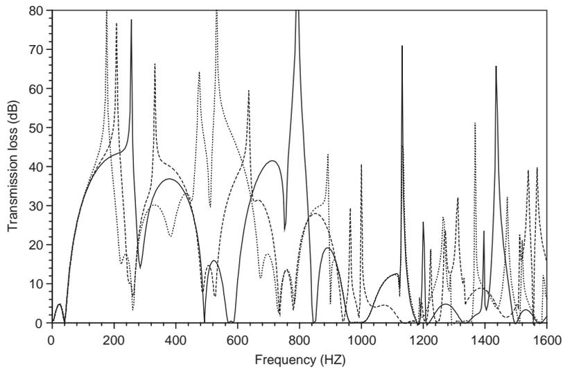
Fig. 5. Effect of location of bulkhead on acoustic attenuation performance of double chamber silencer: ———,  $L_{s1} = L_{s2} = 24''$ ,  $L_{c1} = L_{c2} = 12''$ ; - - - - - ,  $L_{s1} = 27''$ ,  $L_{s2} = 21''$ ,  $L_{c1} = 15''$ ,  $L_{c2} = 9''$ ; ·······,  $L_{s1} = 30''$ ,  $L_{s2} = 18''$ ,  $L_{c1} = 18''$ ,  $L_{c2} = 6''$ .
