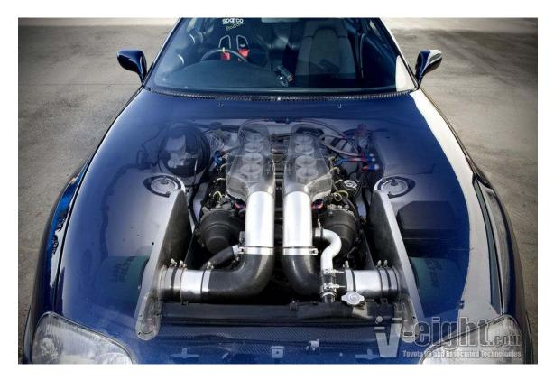
INDUCTION Manifold: Custom Fabricated ITB Manifold Air intake: Twin Custom 4" Filtration system: Uni Filter Inlet pipe: Twin Custom 4" Silicon hoses: 4" Throttle Body (Type/Size): x8 48mm ITB's, modified rb26det units with custom OS butterflies and machined shafts (EFI Hardware) Plenum Chamber: Custom Carbon Fibre Dual Entry Balanced Plenums
