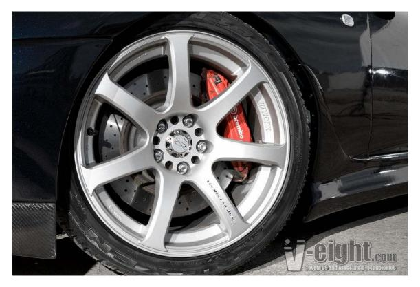
BRAKES Front: 355mm Brembo F50 4 piston calipers on custom brackets Rear: 330mm Brembo GT3 4 piston calipers on custom brackets Booster: Stock Brake pads (F/R): Hawk Lines: TRD
